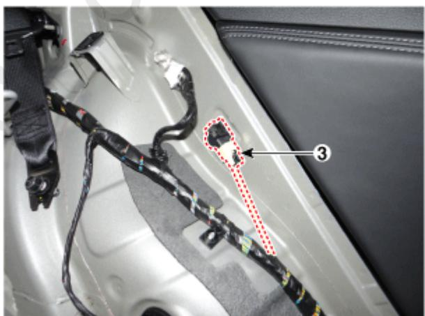
1. Front Pressure Side Impact Sensor (P-SIS)
